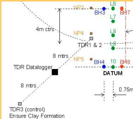
The Time Domain Reflectometry sensors propagate a high frequency transverse electromagnetic wave that is passed through four parallel 'prongs' buried in the soil. They measure the dielectric constant of the soil.
