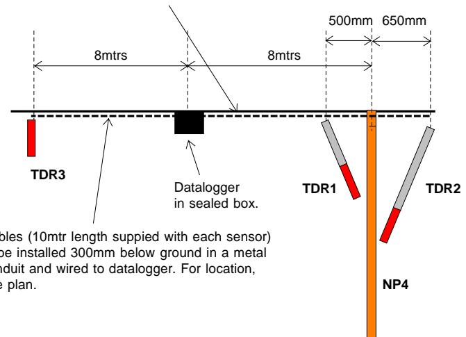
Insert TDR's at an angle, as shown, to avoid accumulation of water in bottom of hole. Apply sealing grout around head of tube and ensure assembly is buried below ground.
