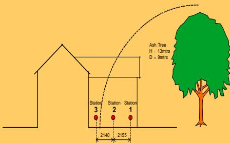
The Ash tree roots took approximately one month before influencing the moisture content of the soil sufficient to cause ground movement 2mtrs along the length of the wall between Stations 1 & 2.
