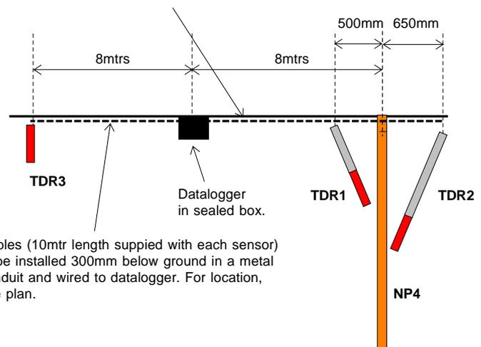
Cables (10mtr length supplied with each sensor) to be installed 300mm below ground in a metal conduit and wired to datalogger. For location, see plan.
