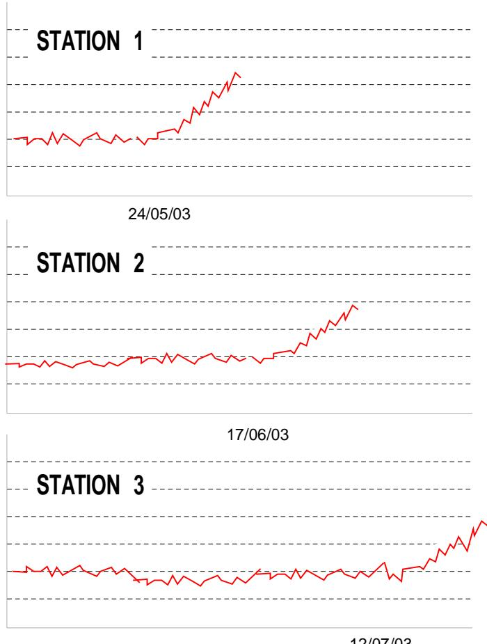
The station nearest the tree (Station 1) registered movement in late May. Station 2 followed less than a month later, and Station 3 registered movement on the 12<sup>th</sup> July. The roots of the Ash tree had changed the moisture content of the soil nearest to the tree first, and furthest away, last.
