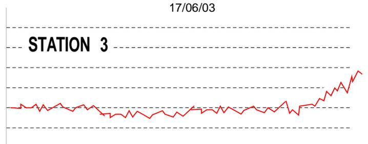
The station nearest the tree (Station 1) registered movement in late May. Station 2 followed less than a month later, and Station 3 registered movement on the 12<sup>th</sup> July. The roots of the Ash tree had changed the moisture content of the soil nearest to the tree first, and furthest away, last.
